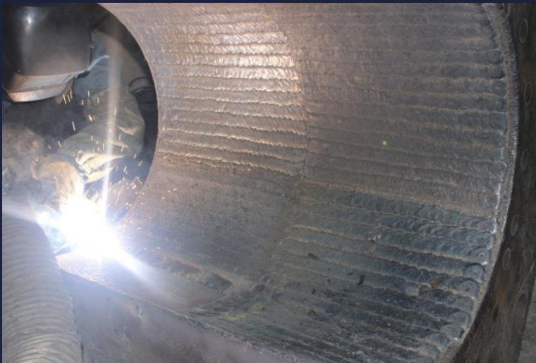
Building-up welding of semi-channel inner surface
