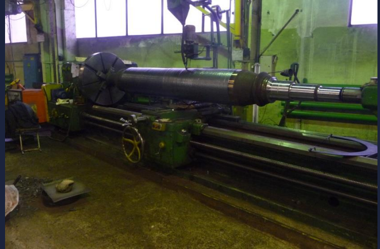
Renovated bearings with babbitt coating
